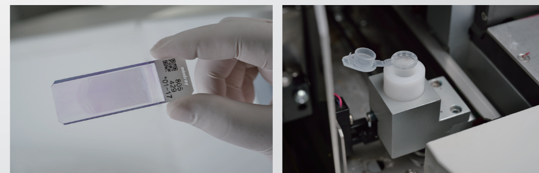
The SC-120 can make smears from capillary samples as it requires only 40µL blood.
